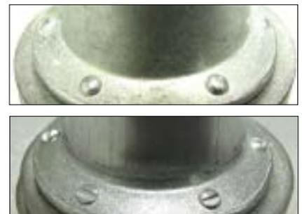
“Dots” on the BobTail collar indicates a full swage when at least one is crossed by the swage anvil.
