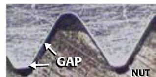
Regular nuts and bolts have gap, which allows for loosening by vibration.
