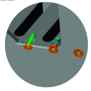
The Visu-Lok® system is a blind fastener that provides high shear, tensile, fatigue, and self-locking capabilities. Unlike conventional nut and bolt combinations, the Visu-Lok blind bolt can be completely installed, and fully verified, from one side of the structure. When installed, the Visu-Lok forms a solid, blind side head, with minimum preload levels guaranteed. Manufactured in 1/16" increments, Visu-Loks have an operational grip range of .062".
