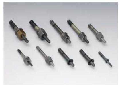
The Accu-Lok Fastening System is designed to be galvanically compati-ble with carbon fiber reinforced composite structures. The main nut body is most commonly made from 6Al-4V Titanium. Alternate materials are available upon request. The sleeve component is made from 300 series Corrosion Resistant Steel. Each assembly also contains a small Acetal
