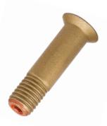
The thread runout on the Aero-Lite® pin is matched to the mating collars, enabling the collars to assemble closer to the full shank of the pins. As a result, Aero-Lite® pins achieve additional grip accommodation in the minimum grip area.
